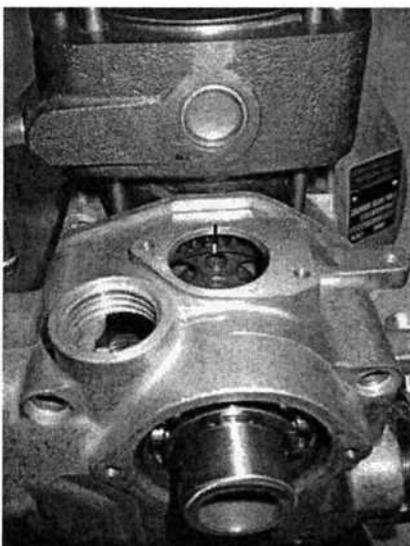
Line up the timing mark on the camshaft gear with the mark on the gear end cover.
