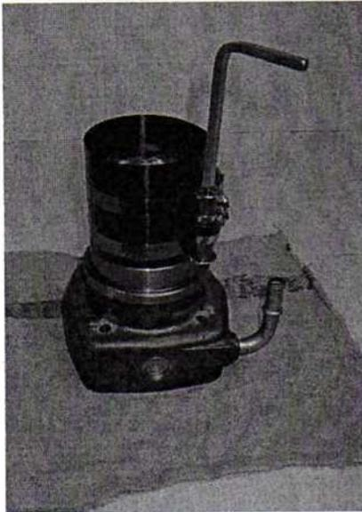
Oil the ring and piston skirts. Check that piston ring gaps are 120 degrees offset. Compress rings with ring compressor. Lay the cylinder down on the bench with bottom facing up. Install piston from bottom side of the cylinder. Never tap on the piston crown.
