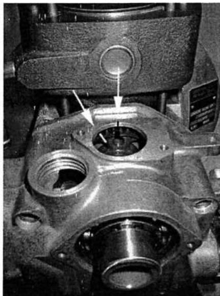
Place new o-ring in the flute of the crankhandle support. Lubricate the camshaft and the sealing lips of the oil sealing ring. Don't push the guide straight onto the gear end cover. Instead use a light twisting motion until the guide seats itself. Tighten the screws to specified torque.
